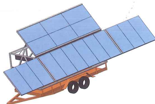
Above is a drawing of NASA's 3kVA photovoltaic power plant. Mounted on a 16-foot trailer, the solar panels span 512 square feet when open and produce three kilowatts of electricity. NASA will use it to test different ways the technology might be used in space.
