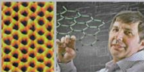
Left: The atoms in a layer of graphene are linked in a pattern like that of chicken wire. Right: Andie Geim, one of graphene’s discoverers
